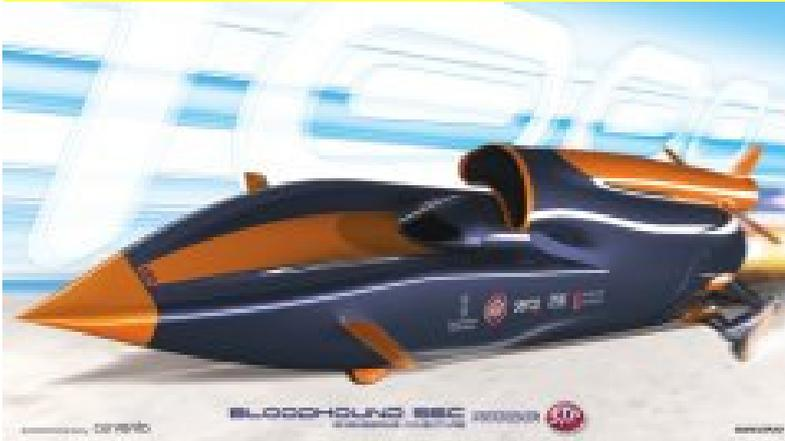
Powered by a Euro-fighter jet engine and a rocket engine producing the combined thrust of 21 tons, equivalent to 140 000bhp, the car will accelerate at 60mph per second, 3g.
